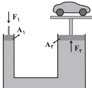
$$\begin{aligned} \frac{F_1}{\frac{\pi D_1^2}{4}} &= \frac{F_2}{\frac{\pi D_2^2}{4}} \Rightarrow \frac{F_1}{D_1^2} = \frac{F_2}{D_2^2} \xrightarrow{D_2 = (D_1 + 1/2)m, F_2 = 18000N, F_1 = 2000N} \\ \frac{2000}{D_1^2} &= \frac{18000}{(D_1 + 1/2)^2} \Rightarrow \left(\frac{D_1 + 1/2}{D_1}\right)^2 = 9 \\ \Rightarrow \frac{D_1 + 1/2}{D_1} &= 3 \Rightarrow D_1 + 1/2 = 3D_1 \Rightarrow 2D_1 = 1/2 \\ \Rightarrow D_1 &= 0.5m = 50cm \end{aligned}$$
